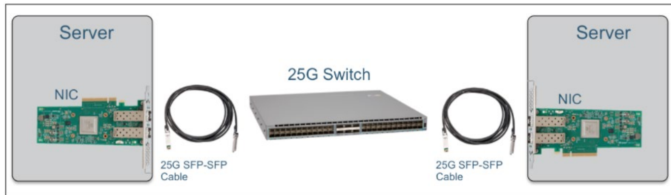
Figure 4: Test set-up for 25G Ethernet Switch-NIC interoperability testing
