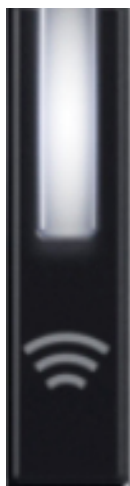
Figure A-3: iDRAC Quick Sync 2 Indicators
